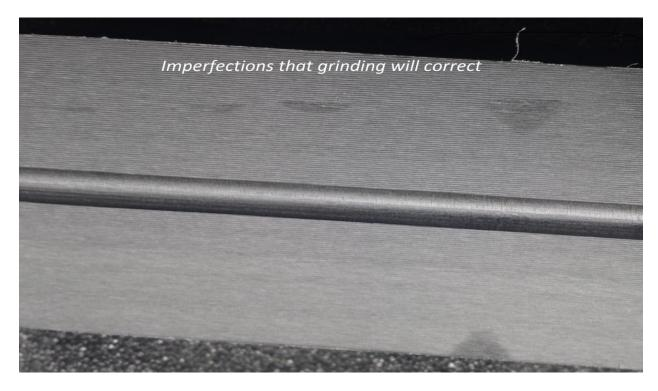
The ski below shows common damage from heating LF4 or similar hardness wax. You can see deformed pockets in the middle of the base and burnt high spots as well. This ski will perform far below expectations BUT can be corrected with stone grinding. These skis were used again last season by a very happy customer!
